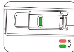
3. When the ISOFIX linker is in the correct installation state , the ISOFIX reset indicator is displayed in green . If the indicator is red , be sure to loosen the connector and reinstall . Push the whole base slowly forward to attach it to the back of the car seat
