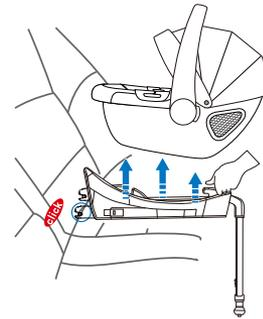
8. Pull the base separation handle, and lift up the handle of the carrier to separate the carrier from the ISOFIX base.
