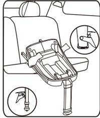
4. Push the ISOFIX base in the direction of the car seat back with both hands at the same time. Make the basket - side against the back of the car seat.
