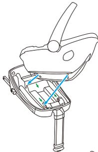
6. The basket ontology slightly back, the shaft into the rear shaft card slot of the base, the rear red and green display green as correct. The front end of the body is rotated into the front axis hook, and the front red and green display is the correct green.
