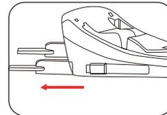
2.Put the ISOFIX base on the car seat, press and hold the ISOFIX unlock button with two fingers at the same time ,and push it outward to the outermost side . Fix the ISOFIX interface on the ISOFIX anchor point on the car until you hear the beep.
